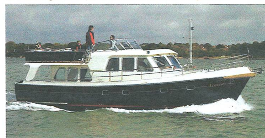
A low coaming and helm position work to keep the air draught down
