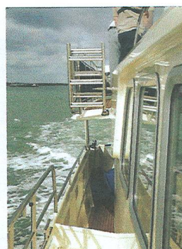
Steps either side hinge clear when not in use, however, they can get in the way
