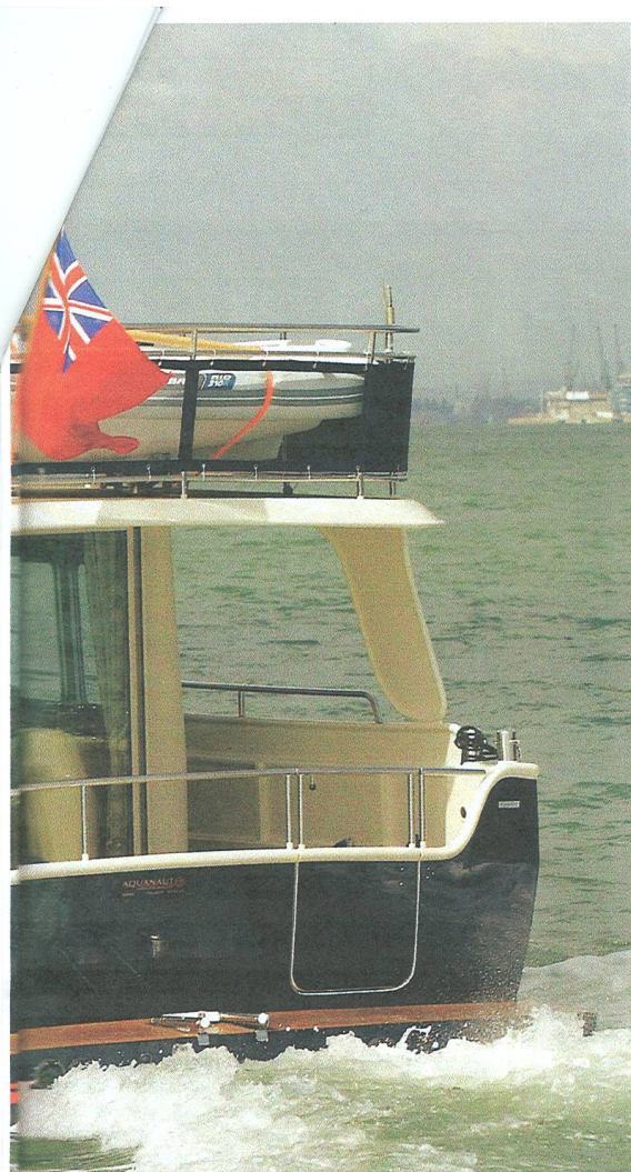
Steps either side hinge clear when not in use, however, they can get in the way
