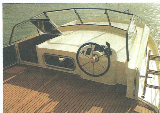
A low coaming and helm position work to keep the air draught down
