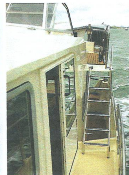
Steps either side hinge clear when not in use, however, they can get in the way
